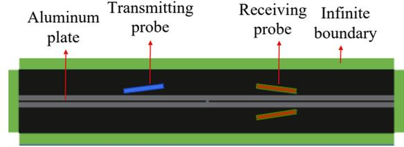
**Fig. 4 Lamb wave propagation simulation model**
