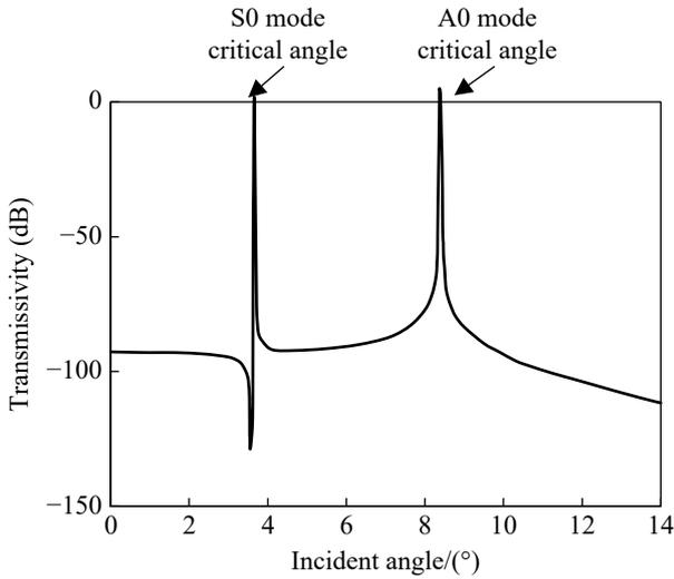
**Fig. 3 Relationship between incident angle and transmittance**
