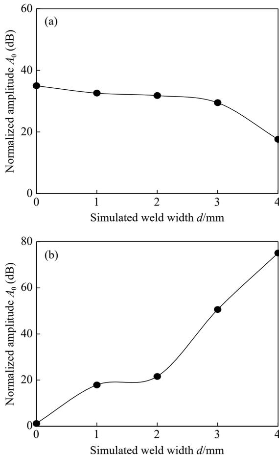
**Fig. 12 Relationship between weld width and amplitude in experiment (a) Reflected leakage wave (b) Transmission leakage wave**
