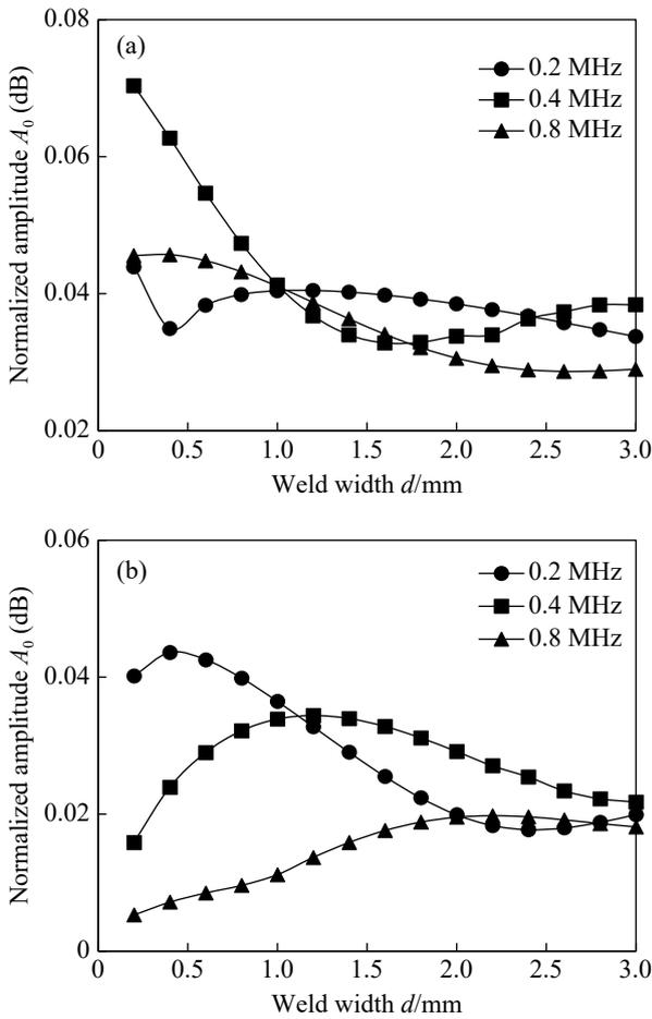
Fig. 8 Relationship between weld width and amplitude (a) Reflection leakage wave (b) Transmission leakage wave
