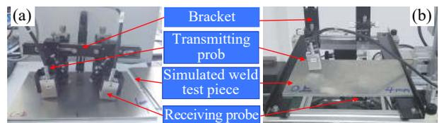
Fig. 11 Schematic diagram of the experimental device (a) Receiving reflected leakage wave (b) Receiving transmitted leakage wave
