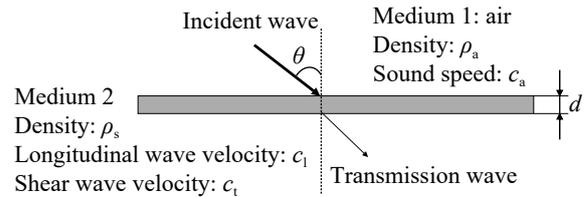
Fig. 2 Oblique incidence of ultrasonic waves in thin plates
