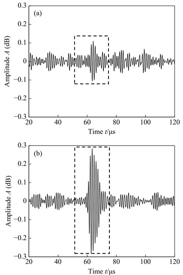
**Fig. 13 The test piece D is used to simulate the good bonding between the weld and the intact part. (a) Not well bonded (Part B) (b) Well bonded (Part A)**
