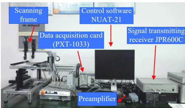
Fig. 9 Air coupled scanning system
